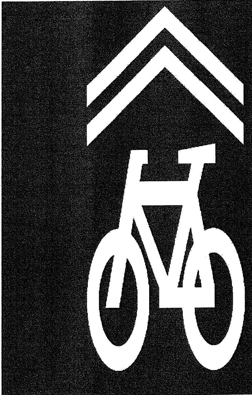
Figure 9C-9. Shared Lane Marking
